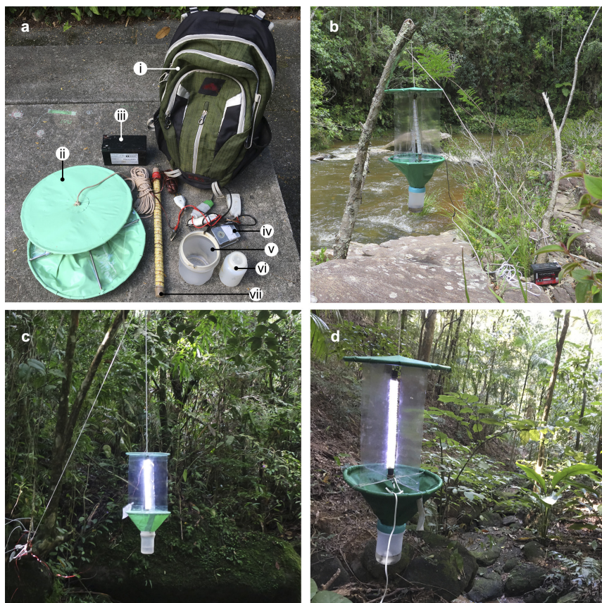
Figure 4. Collapsible Light Trap (CLT) in field. a: Items needed to set up the CLT (total weigh-4.8 kg/steel version, including the backpack) – (i) 35 L backpack to carry all items, (ii) main supports, (iii) 7 Ah 12 V battery, (iv) photo switch (optional) with wire connections, (v) collecting container, (vi) bottle with 300 ml 96% ethanol, (vii) LED light tube; b: CLT set up with tree trunk found near the stream, at Ipoema, Itabira Municipality, Minas Gerais State, Brazil; c: CLT set up at Teresópolis municipality, Rio de Janeiro State, Brazil; d: CLT after collecting night at Tijuca National Park, Rio de Janeiro municipality, Rio de Janeiro State, Brazil.
