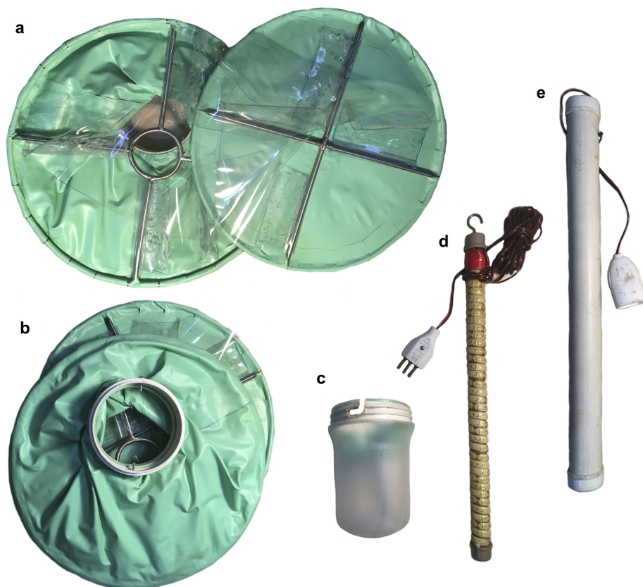
Figure 3. Main parts of the Collapsible Light Trap (CLT). a: main structure, showing the internal metallic supports, both superior and inferior; b: caudal view of the main structure, showing the PVC ring at the opening of the funnel; c: 1 L collecting container; d: LED tube with wire and plug (Brazilian type); e: PVC tube (optional) adapted with a power socket, allowing to connect 8 D batteries in series, to use instead of using an UPS battery.
