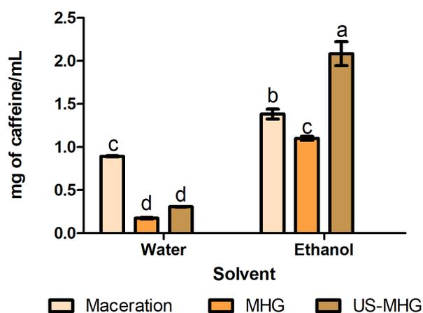
**Figure 2. Caffeine concentration of extracts obtained with different extraction methods. The samples followed by the same letter do not differ by Duncan test ( $p > 0.05$ ). The caffeine content of the two extraction cycles was considered and normalized to 1 mL**
