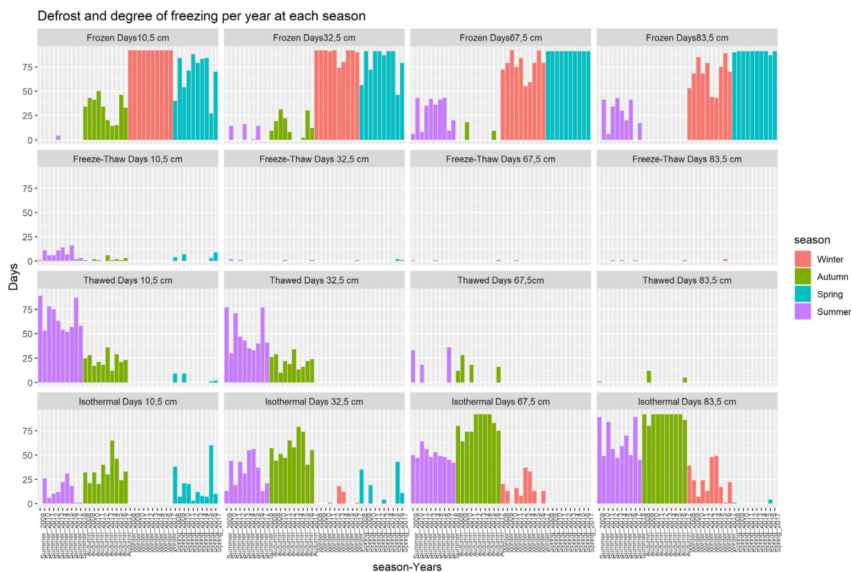
Figure 5. Freezing, thawing, freeze-thawing and isothermal processes by season for 2008 to 2018 for ground temperature at depths 10.5; 32.5; 67.5; and 83.5 cm in Fildes Peninsula - King George Island, Antarctica.
