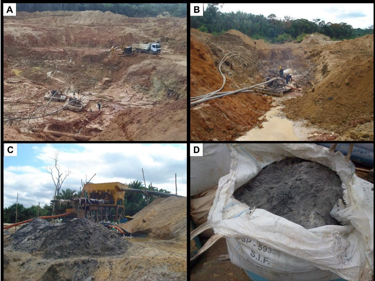
**Figure 2.** (A and B) Overview of the open pit mining of the alluvial Cachoeirinha deposit. (C) Ore concentration equipment gravitational used in Cachoeirinha open pit mining. (D) Bag with ore concentrate for subsequent transport and trade steps.
