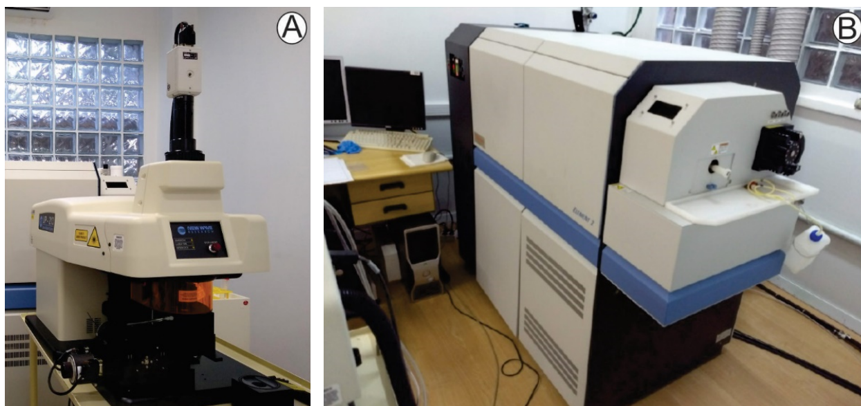
Figure 2. Laser ablation inductively coupled plasma mass spectrometry (LA-ICP-MS) apparatus used in this study; (A) New Wave Research® Nd:YAG deep UV (213 nm) laser ablation system; (B) Thermo Fisher® Element 2 Sector Field ICP-MS.
