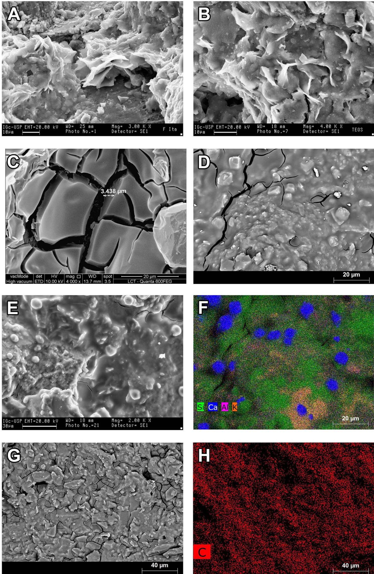
**Figure 11.** SEM images samples of the of Itararé Sandstone treated with swelling inhibitors and consolidant. (A) Porosity of Itararé Sandstone. (B) Montmorillonite covered by TW. (C) and (D) Fractures formed by TW. (E) Sample treated with ATW, showing minor fractures and spheroidal calcium structures. (F) Mapping showing that the spheroidal structures are made of calcium. (G) Image of the sample treated with ATW. (H) Mapping of this area showing a large presence of carbon.
