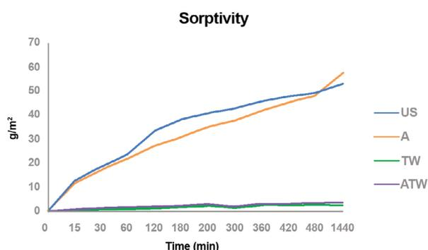
**Figure 9.** Capillarity test in untreated sample, treated with **A**, **TW** and **ATW**.
