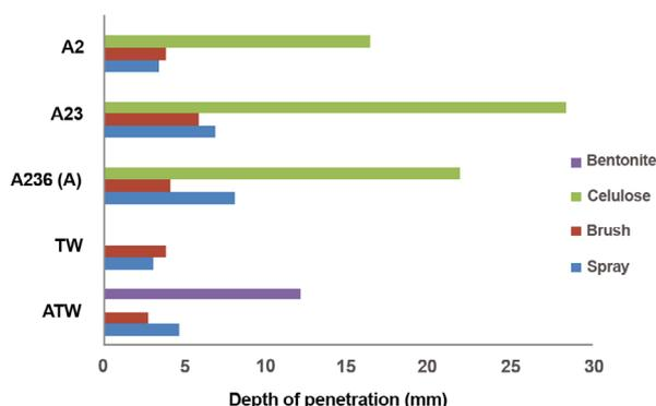
Figure 6. Penetration depth test with different techniques.
