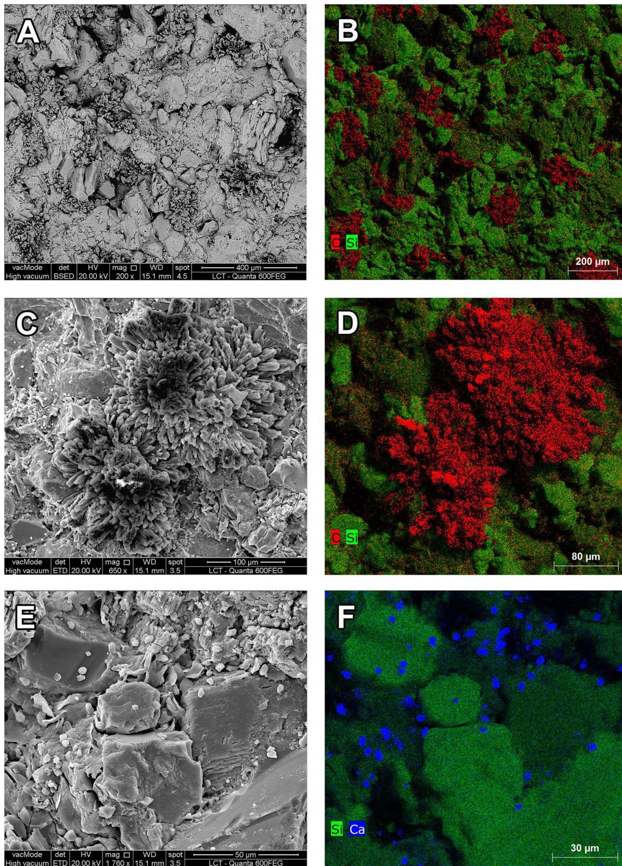
**Figure 10.** SEM images of samples of the Itararé Sandstone treated with swelling inhibitors. (A) Sample treated with A (detail for the flower-shaped structures shown in Fig. 10C). (B) Mapping of Si and C in the same region of Figure 10A, with artificial coloring, showing the carbon flowers. (C) Flower-shaped structures in detail. (D) Mapping of Si and C of the flower-shaped structures. (E) Spheroidal structures made of calcium. (F) Mapping of spheroidal structures.
