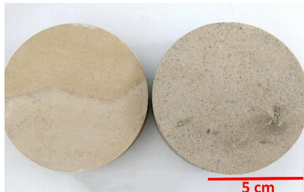
**Figure 2.** Itararé Sandstone, untreated sample.
