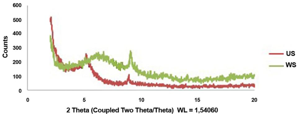
Figure 14. XRD of the untreated sandstone clay fraction (US) and heating-altered sandstone (WS).
