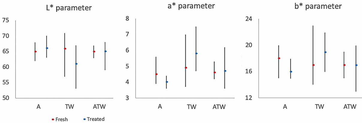
Figure 12. Average of L\*, a\* and b\* parameters for untreated samples and treated with A, TW and ATW.
