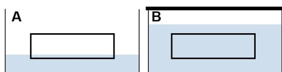
**Figure 4.** Application method of the products. (A) Initially, only the base of the sample was in contact with the product. (B) After the product reached the top by capillarity, the sample was completely immersed in the product.
