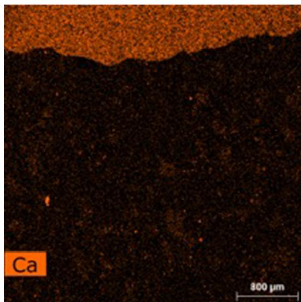
Figure 7. Sample profile treated with **ATW** observed with SEM, showing the presence of calcium inside the stone.
