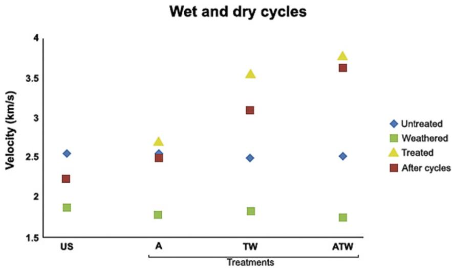
Figure 13. P-wave velocity before and after treatments with A, TW and ATW.
