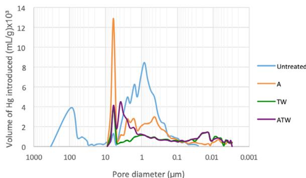
Figure 8. Pore size distribution in mercury porosimetry test in untreated and treated samples **A** (all the three consecutive treatments), **TW** e **ATW**.
