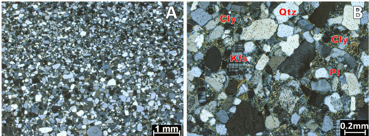
**Figure 3.** Photomicrographs of the Itararé Sandstone. (A) Gradual passage of the thinnest and thickest quartz grains — crossed nicols. (B) Itararé Sandstone mineralogy: quartz (Qtz), potassium feldspar (Kfs), plagioclase (Pl) and clay minerals (Cly) — crossed nicols.
