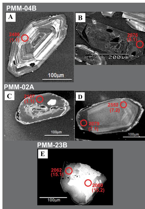
**Figure 7.** Cathodoluminescence images of zircon crystals of the samples (A and B) PMM-04B and (C and D) PMM-02A, with igneous oscillatory and patchy zoning, microfractures, alteration pathways, and metamictic zones. Backscattered electron image of a monazite crystal of sample PMM-23B with (E) convolute zoning. Crystals showing their respective SHRIMP spots (spot number) and  $^{207}\text{Pb}/^{206}\text{Pb}$  ages in Ma.
