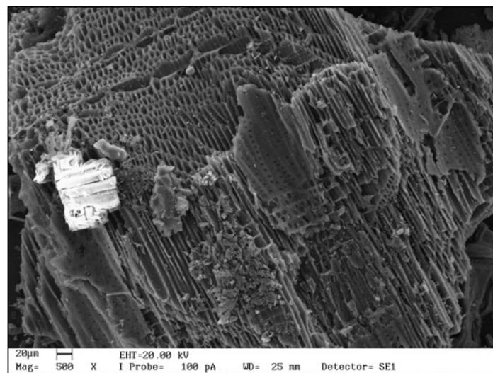
**Figure 1.** Scanning electron microscopy of eucalyptus biochar (magnification of 500×).
