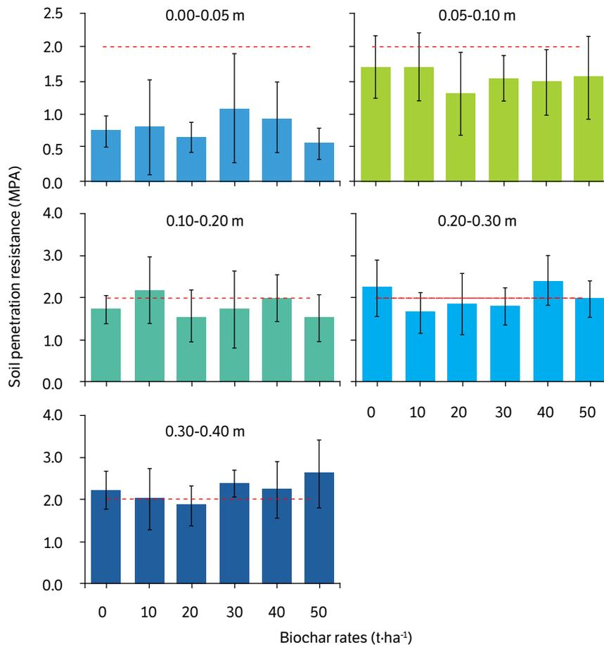
**Figure 5.** Soil resistance (layers 0.00–0.05; 0.05–0.10; 0.10–0.20; 0.20–0.30; and 0.30–0.40 m) after 28 months of application of doses of biochar equivalent to 0, 10, 20, 30, 40 and 50 t·ha<sup>-1</sup>. Equilibrium soil moisture after being submitted to -0.033 Mpa·m. Limiting value for the growth and development of root systems (Tormena et al. 1998). Bars indicate de standard deviation (n = 4).
