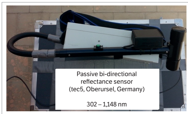
Figure 1. A passive bi-directional reflectance sensor measuring wavelengths between 302 and 1,148 nm.
