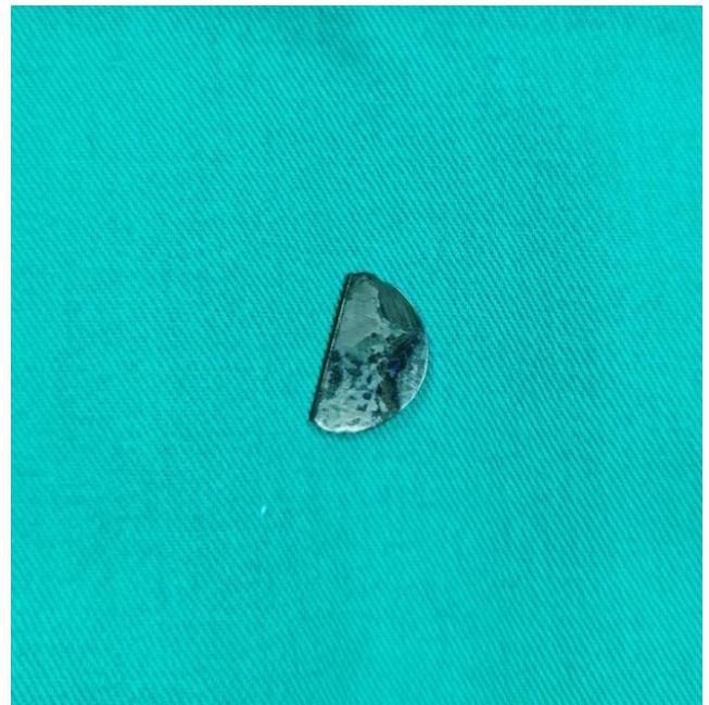
Fig. 2 - Extracted mechanical valve hemidisc.
