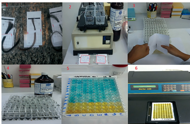
Subtitle: 1. Separation of hair samples; 2. washing of samples; 3. cutting; 4. addition of isopropyl alcohol; 5. addition of chemical reagents; 6. time to read the plates.
